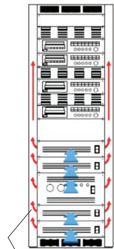
airflow out equipment sides not “choked”
