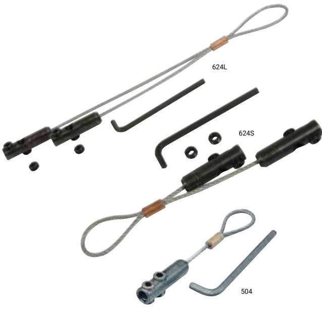
Each grip has two opposed set screws that provide positive locking. Openings in wire grip should be 50% filled with wire to assure slip-proof grip.
