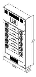
Layout F: Bottom-Fed Pow-R-Line CS Main/40X Distribution (1200A Maximum at 600 Vac)
