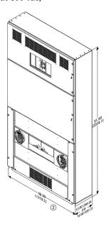
Layout D: Bottom-Fed CMP-A2 Main/PUC/21X Distribution (1200A Maximum at 600 Vac)
