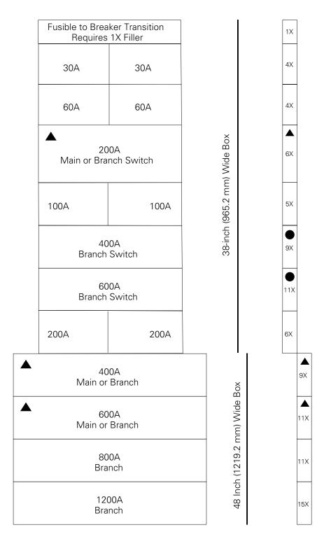
Figure 2-7. Branch and Horizontally Mounted Main Device Layout — PRLCS
