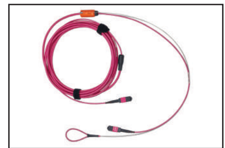
FM4MMB1010M, FX MPO Trunk, OM4, MPO-12 (Male to Male), Type-B, 1 x MPO-12 (12 fibers), 10 m, OFNP, Mini-Distribution 4.8 mm (Double-Jacket), Erika Violet Jacket
